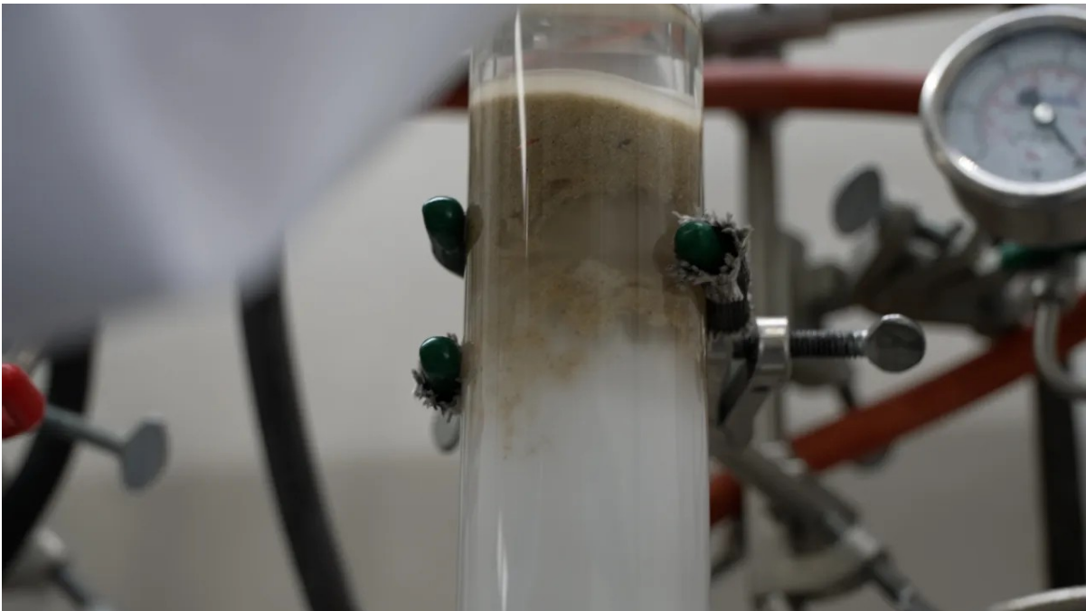
A solvent carrying rare earth elements passes through a filter. (Eric Henrikson/KXAN)
